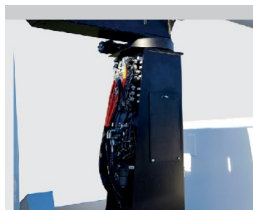
Ground level emergency lowering from the load area (pedestal mounted valve bank)
