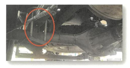
Versalift ask, that in the first instance, end users inspect the U-bolt clamps to ensure they are secure and that the bolts have not loosened (the torque values for these bolts is 68Nm). If the bolts/ clamps are found to be loose then all work(s) must be stopped and Versalift informed.
