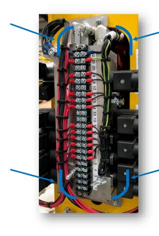
This may be attributed to vehicle/ lift mistreatment and misapplication such as overloading however, Versalift ask that in the first instance the end users inspect the areas shown to the left for damage before use.
