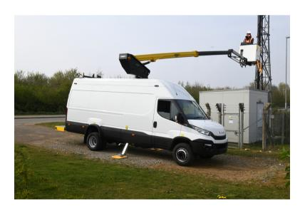
Ideally suited for motorway and dual carriageway use, the VTM-170-F is equipped with intuitive LMC load sensing providing variable outreach based on pressure in the boom lift cylinder. Other features include zero tail swing - even with A-frame outriggers deployed – and the choice of walk-in or duck-under bucket.
