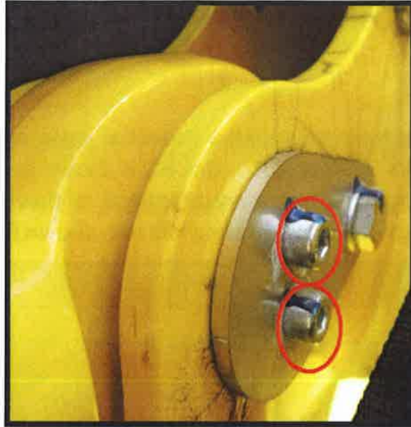
Figure 3: Pear shape washer location at lower end of compensating link.
