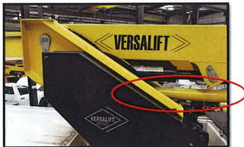
Figure 1: LAT-160F Compensating link location.
