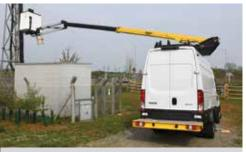
Impressive outreach with LMC load sensing system. A-frame outriggers and tail swing of turret within the mirrors of the vehicle for improved safety.
