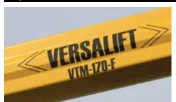
Manufactured from ultra-high strength steel, a profiled boom delivers exceptional rigidity, strength and smooth platform operation. For low maintenance, integrated boom wear pads now follow this profile.
