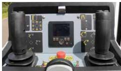
Optional twin joystick IPC control system enables load dependent variable outreach and up to two actions simultaneously.
