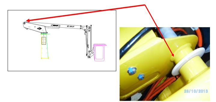
The bosses concerned are welded to the sideplates of the main boom fabrication. However, please note that weld undercut or cold lapping can often be mistaken for a crack and any concerns can be clarified by the use of Dye Penetrant Inspection (D.P.I) techniques.
