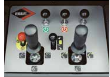
Easy to use fully hydraulic proportional control
