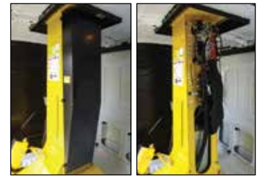
Emergency lowering valves located in pedestal within load area are safe and easy to access
