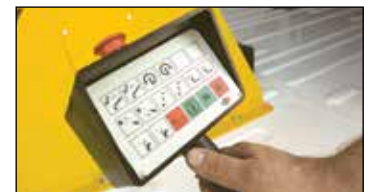
12V DC emergency ground controls
